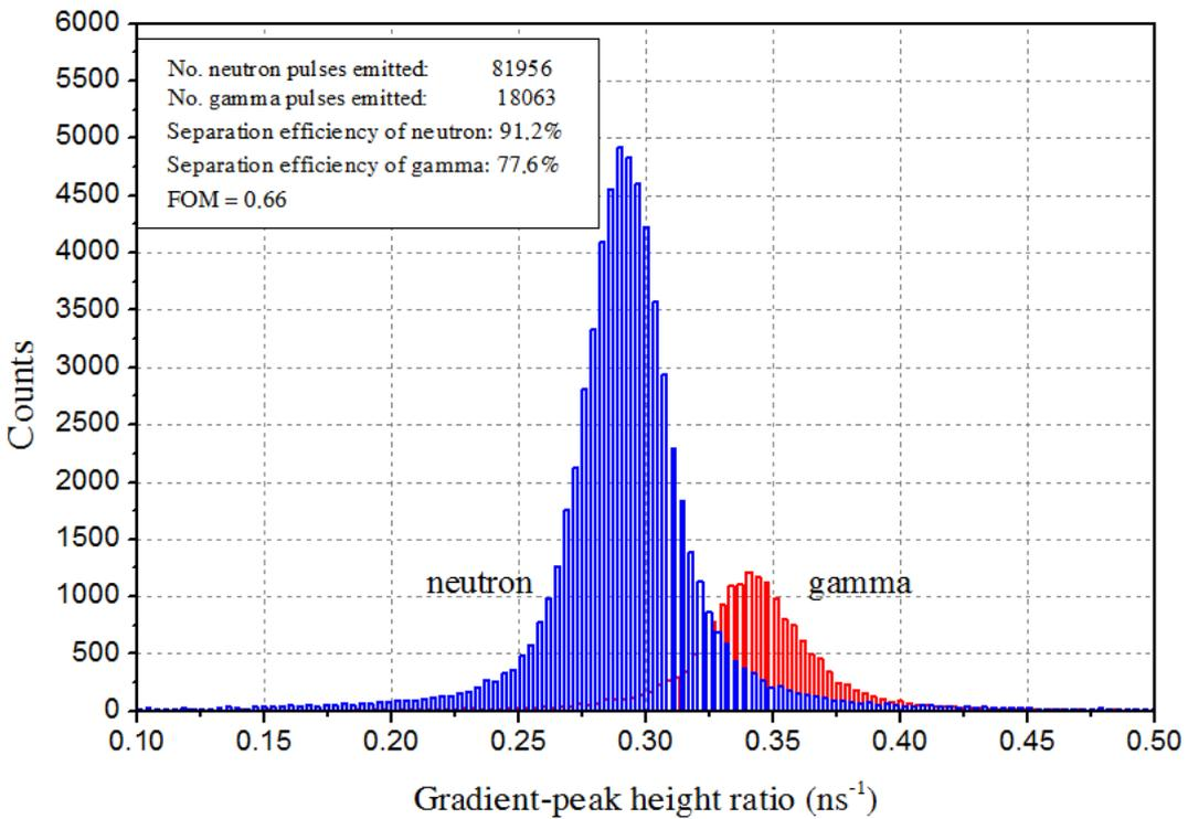
**Fig. 10.** Histogram of pulse gradient analysis.
