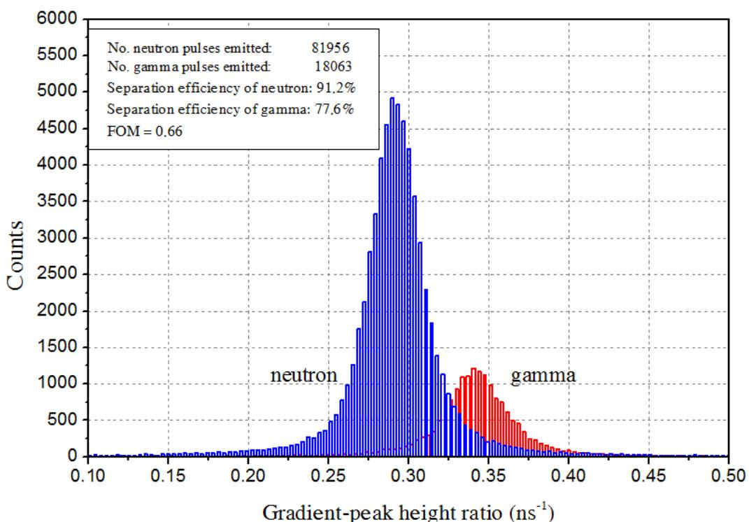
**Fig. 10.** Histogram of pulse gradient analysis.
