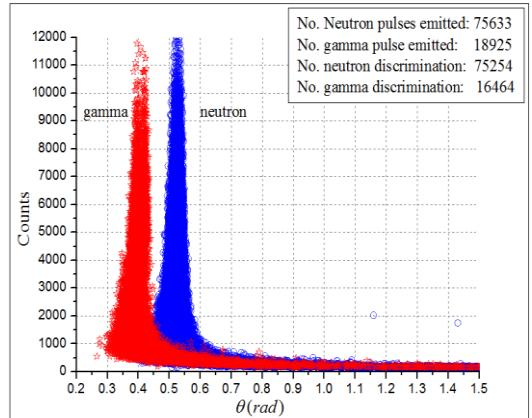
**Fig. 8.** Angle ratios versus pulse heights.
