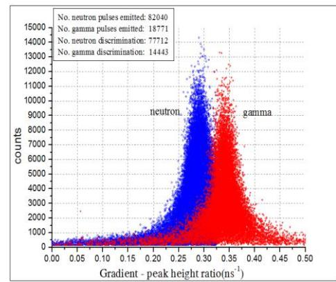
**Fig. 6.** Gradient to amplitude ratios versus pulse heights.
