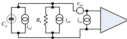
Fig.2. Equivalent circuit for noise analysis.
