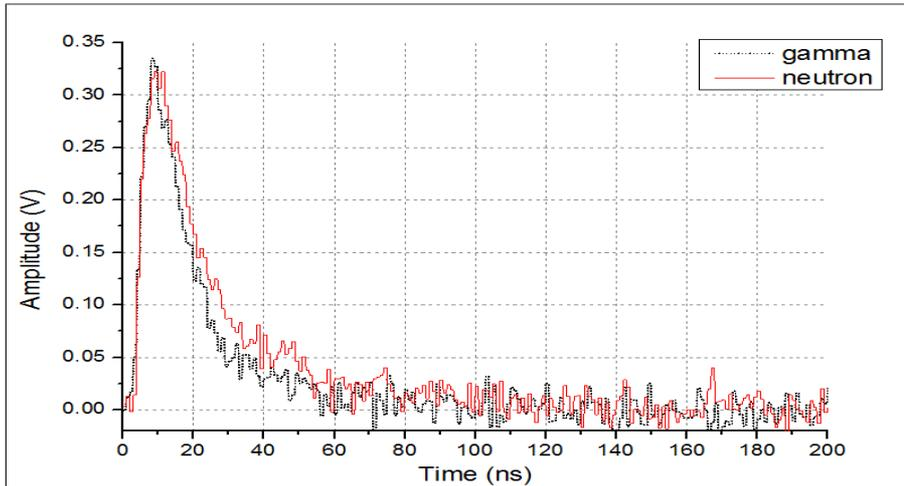
*Fig.3. The simulated pulse for NE213 detector.*
