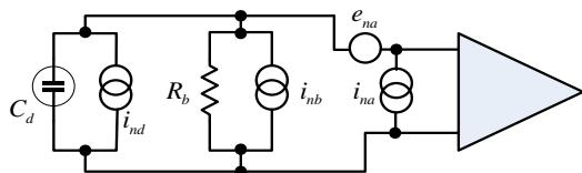
**Fig.2.** Equivalent circuit for noise analysis.
