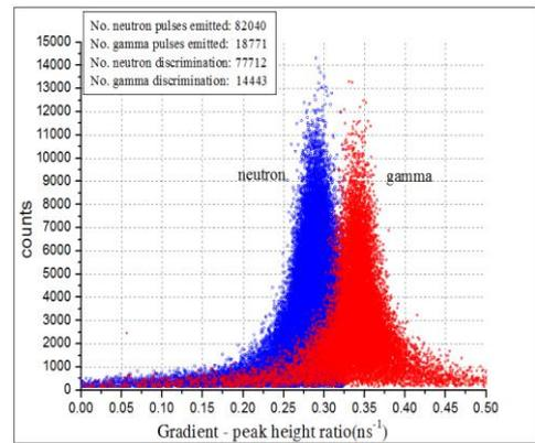
**Fig. 6.** Gradient to amplitude ratios versus pulse heights.
